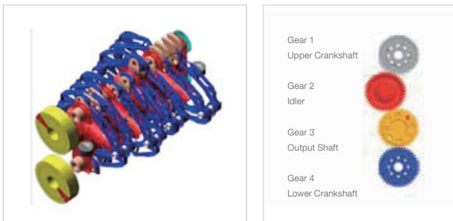
Figure 1: FEV Virtual Engine (powered by Adams) Crank Train model with Flexible Components and Rear View of the Gear Train
